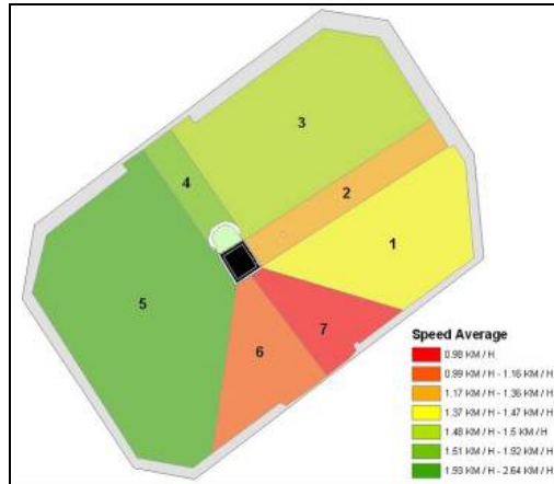
Figure 13. Color-coded map showing the pedestrian average speed at different zones in the courtyard.
